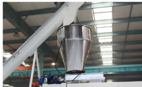
Dosing feeder unit
